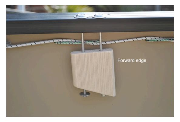
You now need to determine the length of the cross bar, remembering to take your measurement from the bottom of the riser blocks, allowing for some excess on either end and then cut to length. Using the same technique mentioned above mark out the location of the holes in the cross bar. When drilling the holes remember that they will need to be at an angle (appprox 15-20 degrees) to allow for the bolts to pass through the angled cross bar.
