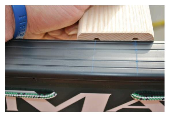
Using a riser block to check the location of holes.
