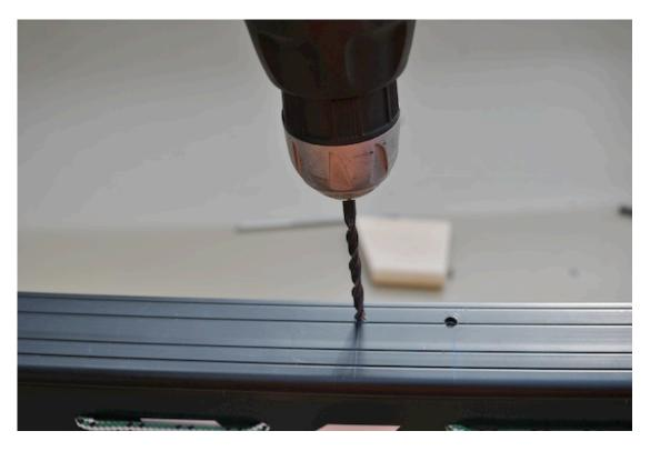
Remembering to measure twice and drill once repeat the procedure on the opposite side. Once completed fit your riser blocks in position, up the correct way and with the longest edge towards the front. This will allow you to check their position and help you with determining the correct length to cut the bar.
