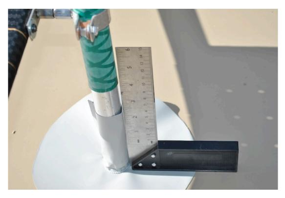
I particularly like the vinyl mast foot as it folds flat when loaded with kit or when the seat area is being used. Generally I position the mast foot etc in the area to the rear of the front seat. Note the removable bracket I have used on the seat to hold the mast securely and the setsquare I have used to ensure everything is square.
