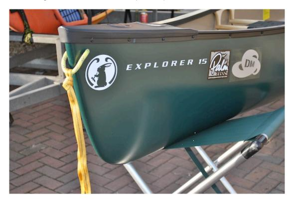
The finished article above with the swim tail fitted. Note the small size of the grab loop. If you are going to attach painters remember that they go through this loop, and can be either permanently attached or removable for transporting. As for length then it is again very much down to personal choice and how/where you will be using your boat. I would suggest as a minimum, a boats length of floating rope. If you choose longer then consider how you will
