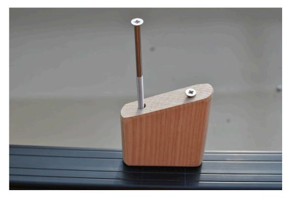
Now using the riser block again, but upside down and making sure it is flush with the inside of the gunwale, I start to screw the supplied bolts in. When I then remove the blocks I will have the position of the holes marked and ready for drilling.
