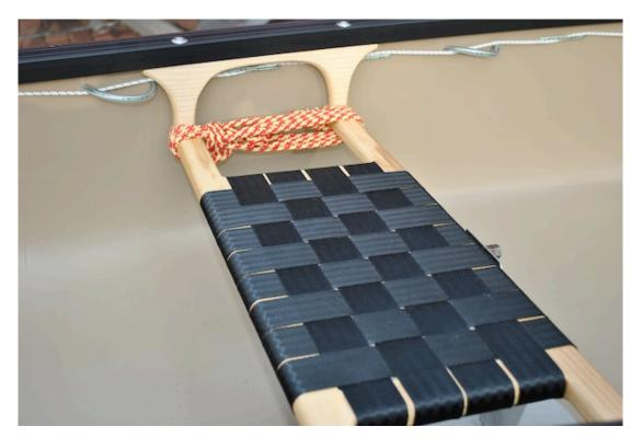
Once I've completed both sides I use 5mm shock cord and weave this through the loops on the inside, as in the photo above. This adds a convenient and secure way for storing things that I may want to access quickly like my sponge or the grip on a paddle.
