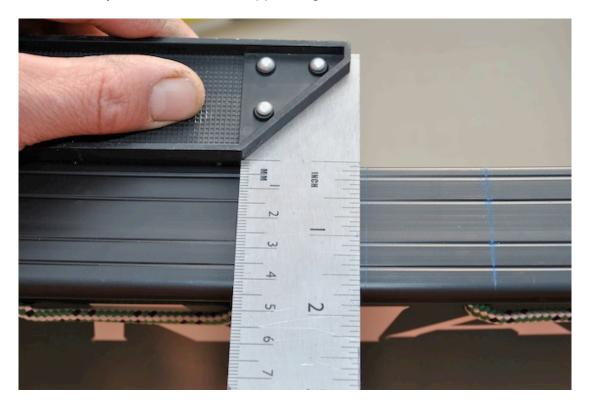
Above using a setsquare to mark my holes prior to drilling.
