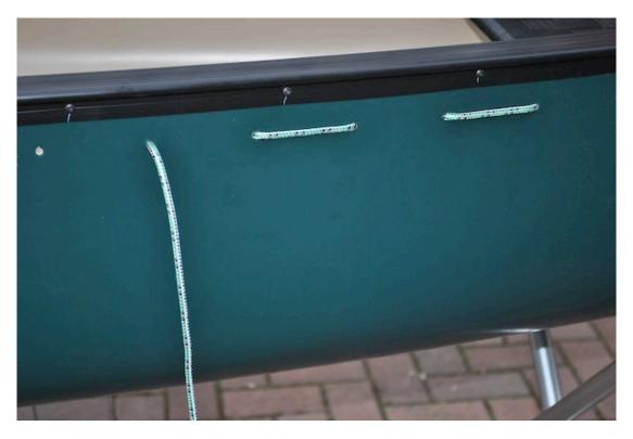
I used a 5mm drill bit so that the cord (also 5mm) is a snug fit. With the holes drilled I start at one end, and secure with a knot on the inside then begin to lace down the sides of the boat using 5mm cord. I personally would not use anything less than 5mm cord for the lacing as it could slice through the plastic like a cheese wire.
