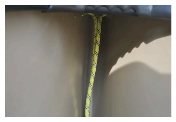
Once drilled and cleaned out, thread your rope through so that both ends of the rope end up inside of the bow and below the deck plate.
