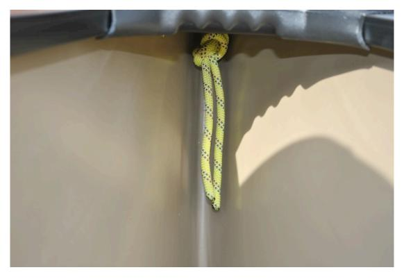
At this point I make sure that the loop on the outside is snug to the hull before tying a overhand knot on the bight close up to the inside.
