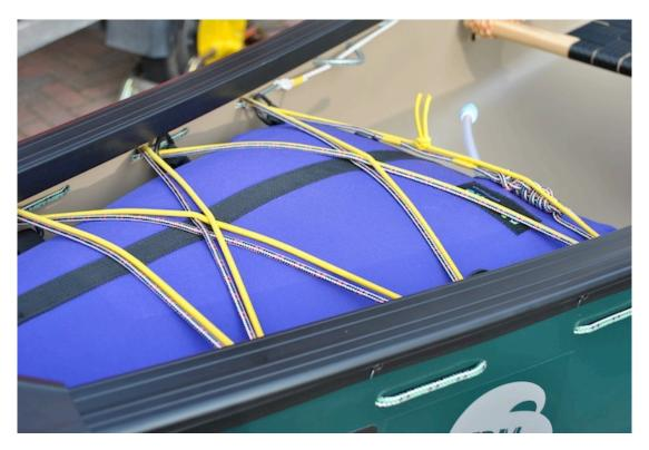
I have also added some shock cord over the bags for tucking a spare paddle and swim lines etc under. Note I don't recommend using only shock cord to secure your airbags, as this will allow too much movement in the bags, possibly resulting in the air bag being popped out when swamped.
