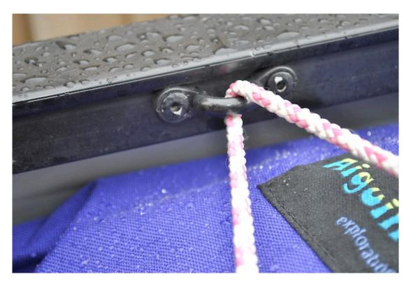
Above an example of a P-clip with cord lashing and a protective air bag cover visible.
