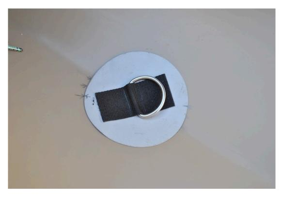
I use my inflated air bags to work out exactly where I want the rings and draw round them. I have used large 2" rings for this job. Note the angle I have had to set the rings at in order to accommodate the shallow 'V' of the hull.
