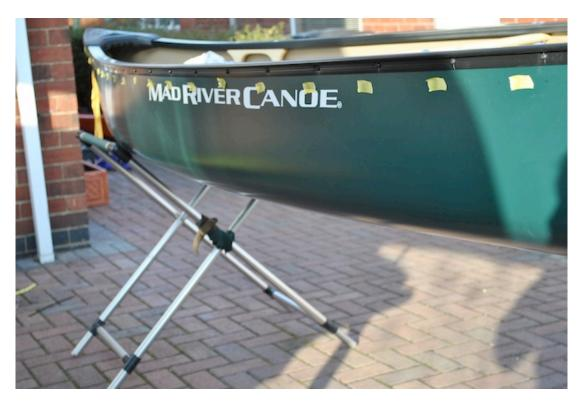
As I intend to lace the entire length of the boat I start at the centre of the boat marking holes either side of the ends of the Yoke. I then continue this process down both sides of the boat and to each end marking where the cord loops will be on the outside with yellow tape. Remember to make sure that the end of the cord should end up inside the boat at the last hole.
