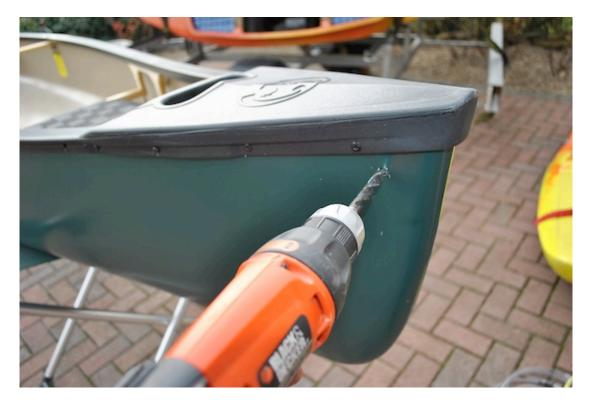
Start by drilling a hole just large enough for your rope on either side at both the bow and stern. I have chosen to drill my holes around 6-8 cm back from the bow and 6cm down from the top of the deck plate. At this point remember the old adage, measure twice, drill once! Or in my case measure, measure, measure and then measure some more before taking a deep breath and drilling!
